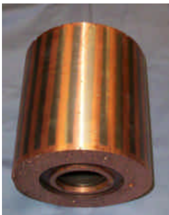
Figure 8. Photograph of die-cast copper rotor turned on the OD to expose the conductor bars. Trapped air bubbles are not seen in the bars but are clearly visible in the end ring.
