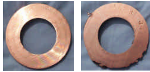
Figure 9. Photographs of sectioned end rings with 55% pre-fill. Ejector end rings on left; gate end rings on right.
