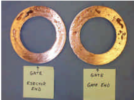
Figure 7. Photographs of sectioned end rings from copper rotors typical of baseline die casting conditions.
